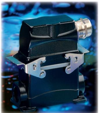
Series B HT housings are made of sea-water resistant die-cast aluminium alloy. The seals are made of Viton and are temperature resistant up to 200 °C. The locking levers are made of stainless steel.
