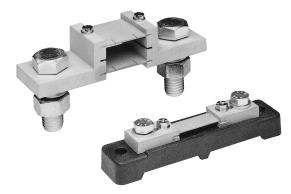
Designed and manufactured to comply with the requirements of DIN43 703 this range of shunts provides an accurate D.C. millivolt signal, exactly proportional to the system current, to drive ammeter indicators, overload protection and control devices.
